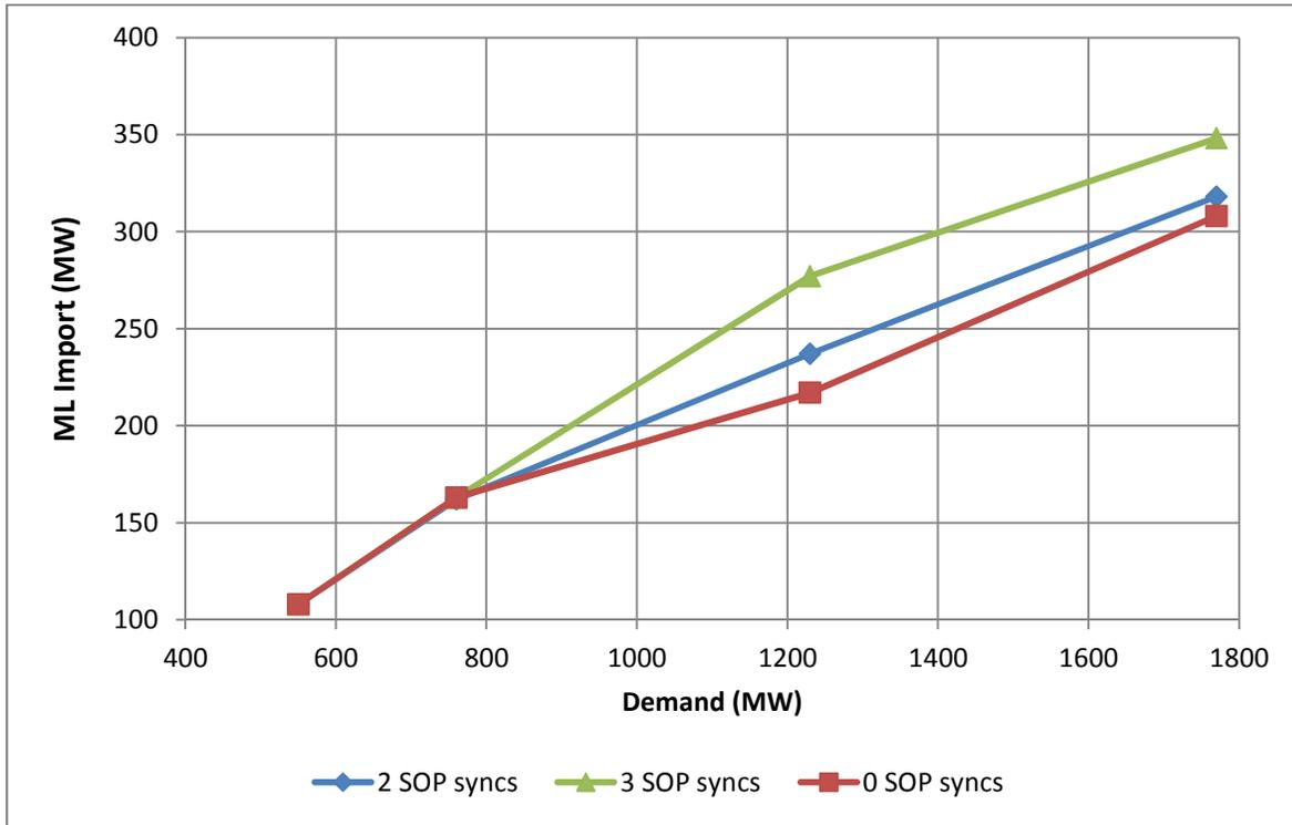
Figure 8-1. Maximum ML import levels – 2 (blue), 3 (green) and 0 (red) SOP synchronous
