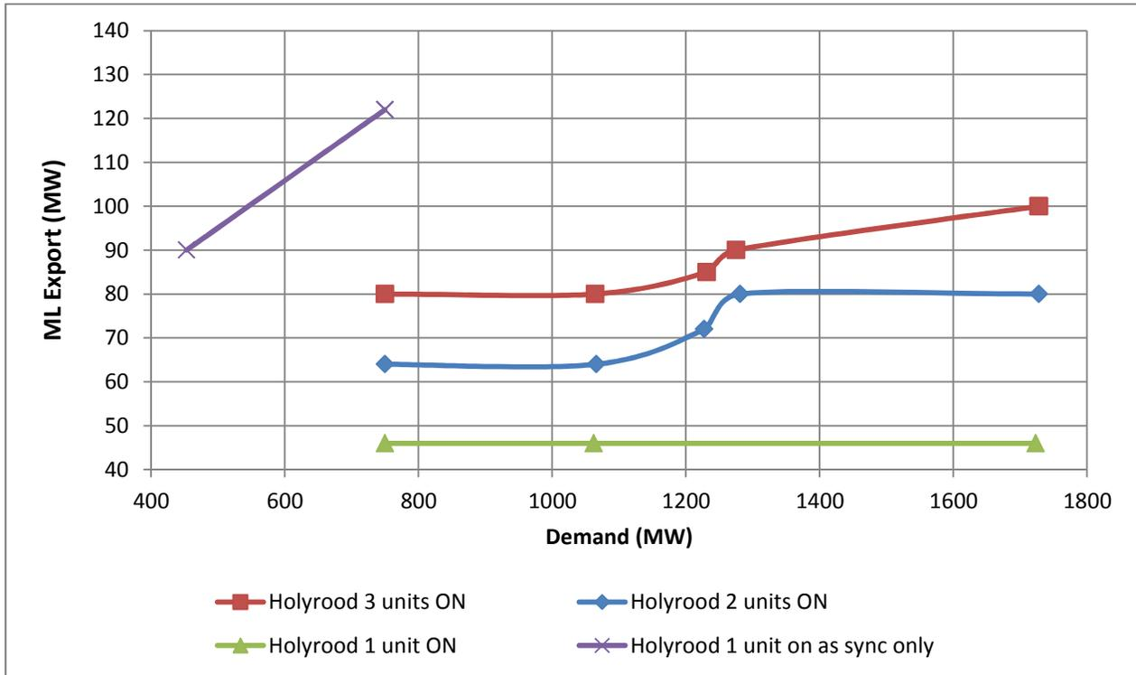
Figure 5-8. ML export limits, 3 SOP synchronous condensers in-service
