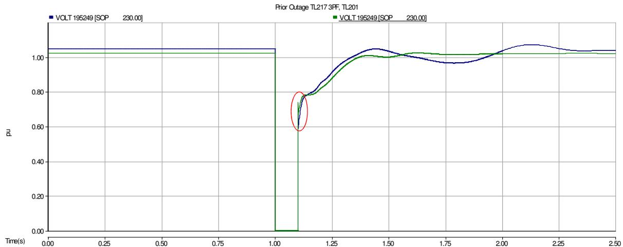
**Figure 6-1. Prior outage TL217. 3PF at SOP on TL201. With 2 SOP syncs (green), and with 0 SOP syncs (blue).**
