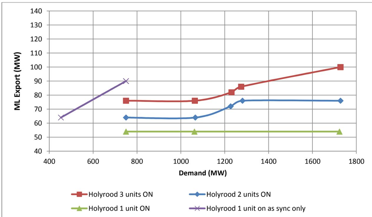
Figure 5-9. ML export limits, 0 SOP synchronous condensers in-service
