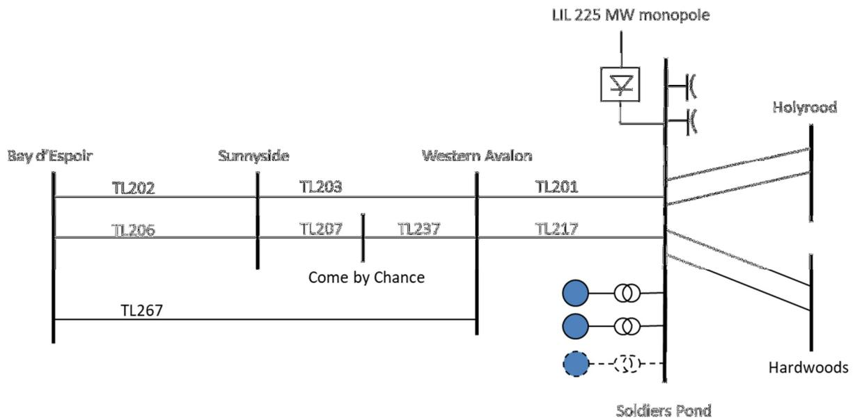
**Figure 5-1. 230 kV transmission corridor from BDE to SOP**
