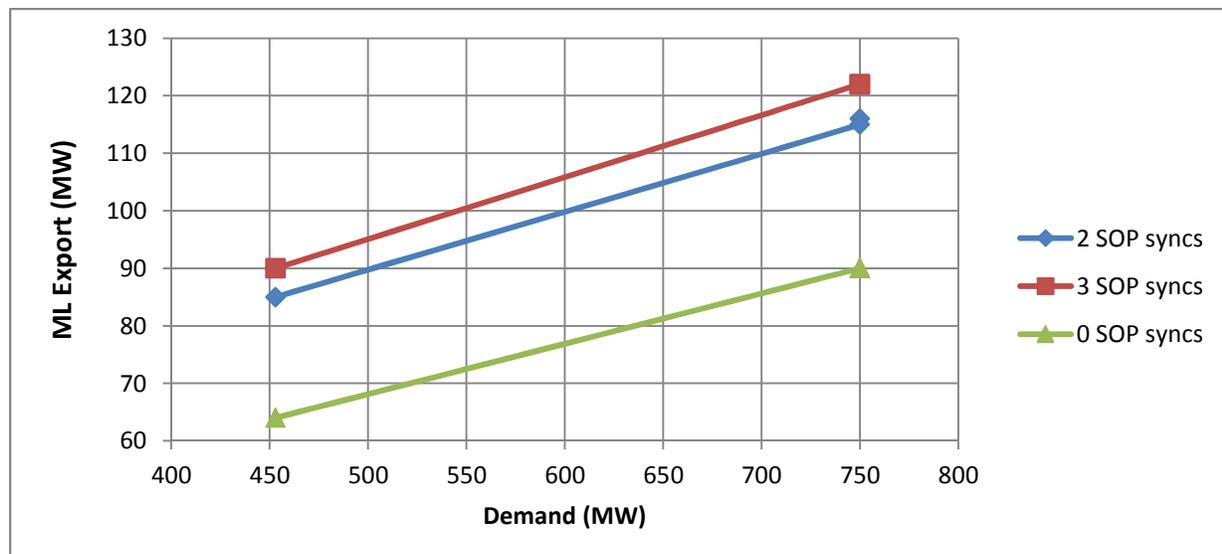
**Figure 1-2. Island demand < 750 MW. Maximum ML export levels - 2 (blue), 3 (red) and 0 (green) SOP synchronous**
