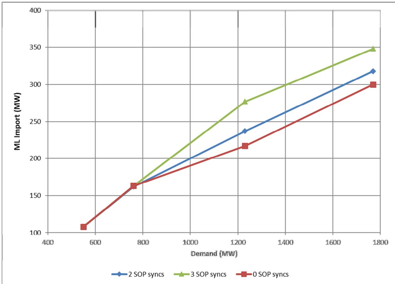
**Figure 5-6. Maximum ML import levels – 2 (blue), 3 (green) and 0 (red) SOP synchronous condensers in-service**
