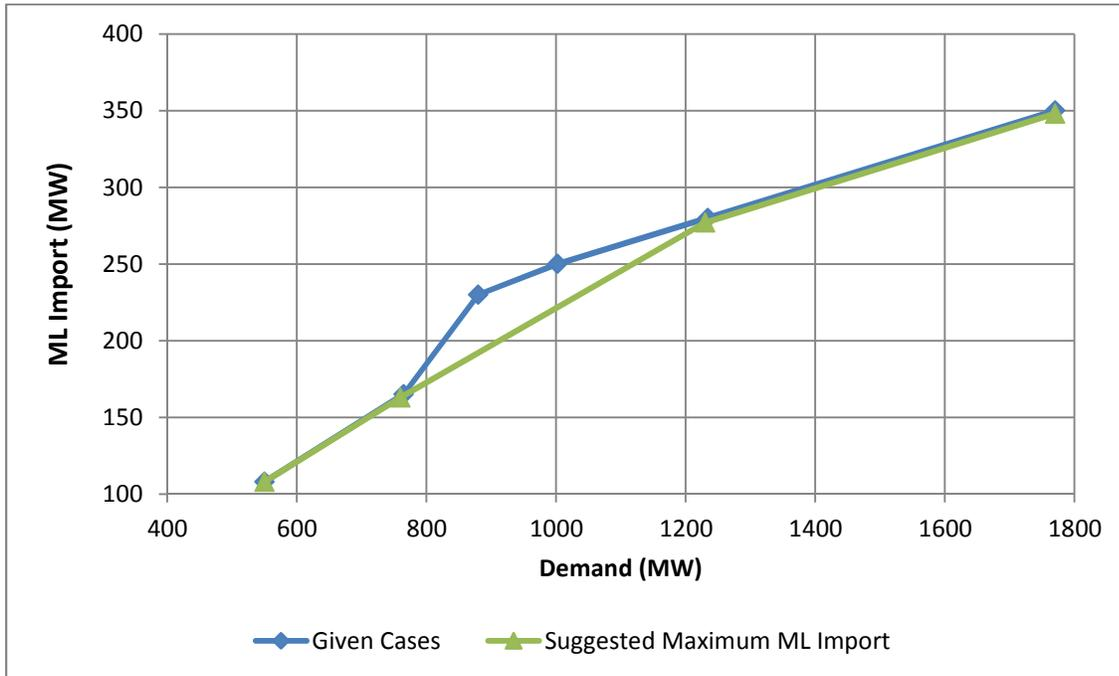
**Figure 5-4. ML import limits, 3 SOP synchronous condensers in-service**
