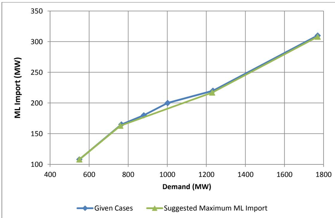
**Figure 5-5. ML import limits, no synchronous condensers in-service**
