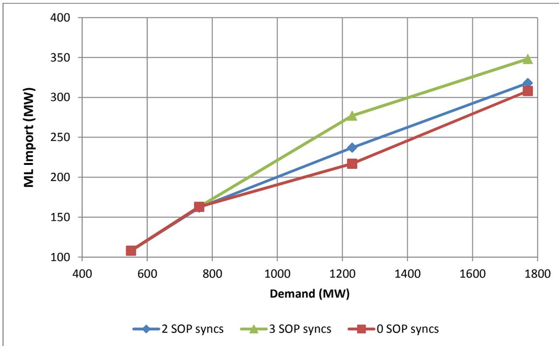
**Figure 1-1. Maximum ML import levels – 2 (blue), 3 (green) and 0 (red) SOP synchronous condensers in-service**
