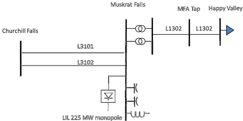
**Figure 3-2. Labrador system near Muskrat Falls**
