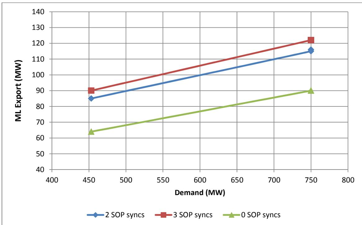
Figure 8-2. Island demand < 750 MW. Maximum ML export levels – 2 (blue), 3 (red) and 0 (green) SOP synchronous
